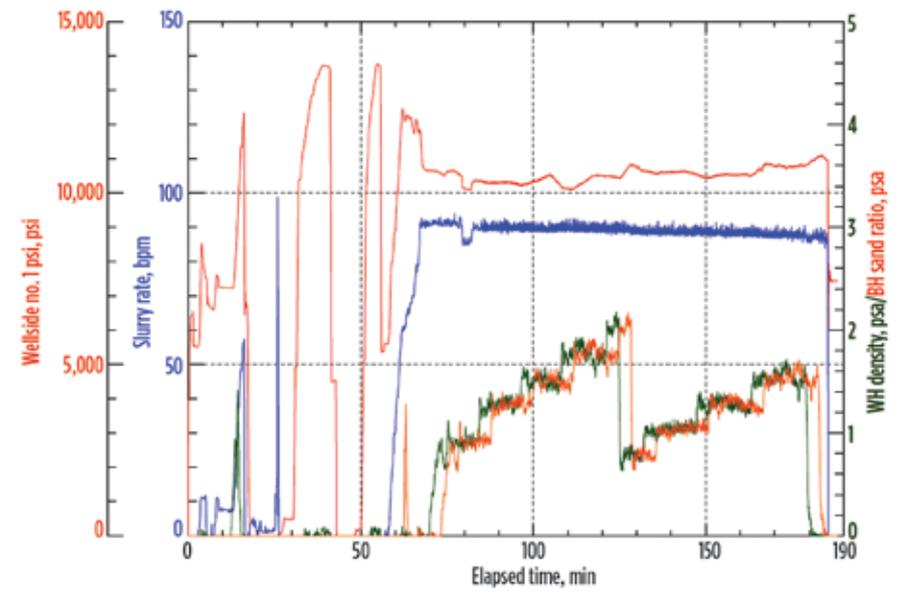
**Fig. 2.** A conventional friction reducer pumped at a 1-gpt minimum and adjusted to as high as 1.2-to-1.3 gpt. ThinFrac MP was added for extra viscosity, when needed.
