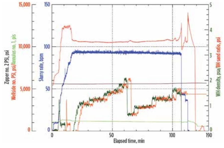
**Fig. 4.** ThinFrac MP pumped at 0.5 gpt, achieving an average 3 bpm more throughout the stage. Similar surface treating pressures were observed.
